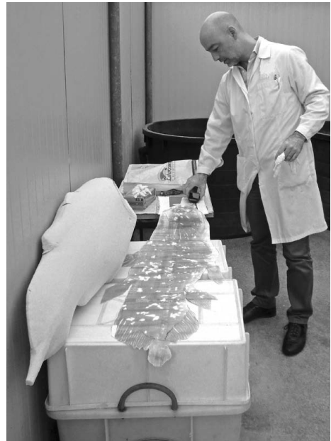
Fig. 3 – Sculpture phase of a polyurethane manikin created on a template paper at scale 1:1.
